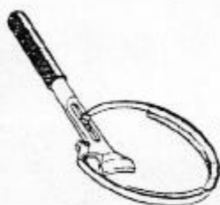
09927 — 56020 Crankshaft pulley holder
