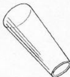
09926 — 18210 Oil seal guide(vinyl resin)
